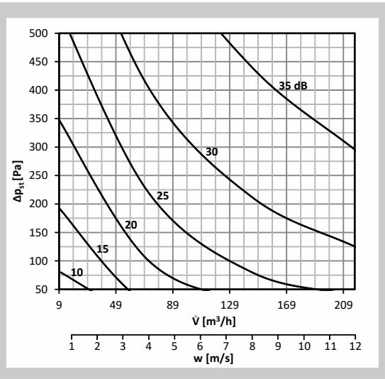
**Graph 26** Sound power level LWA [dB(A)] radiated outside the pipeline DN100, with insulation
