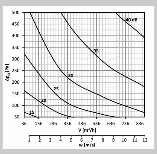
**Graph 30** Sound power level LWA [dB(A)] radiated outside the pipeline DN180, with insulation
