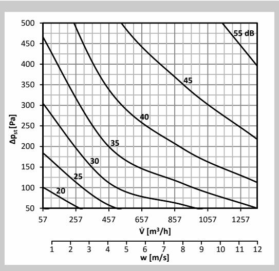
**Graph 21** Sound power level LWA [dB(A)] radiated outside the pipeline DN225, without insulation
