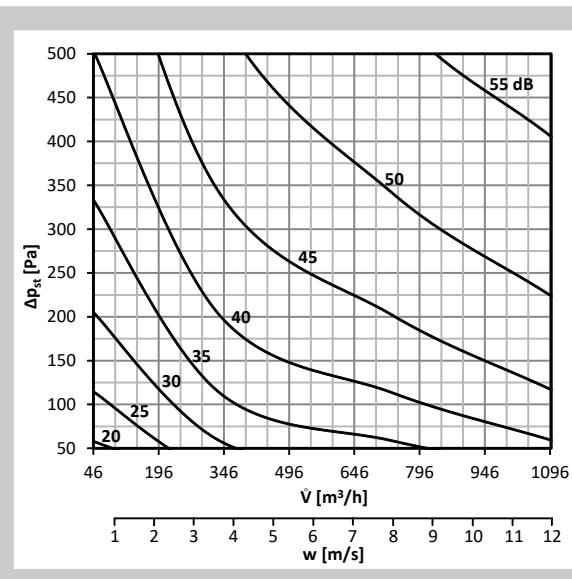
**Graph 20** Sound power level LWA [dB(A)] radiated outside the pipeline DN200, without insulation
