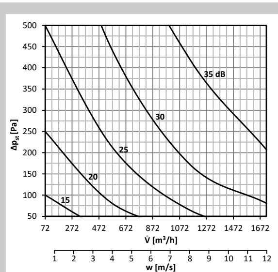
**Graph 33** Sound power level LWA [dB(A)] radiated outside the pipeline DN250, with insulation
