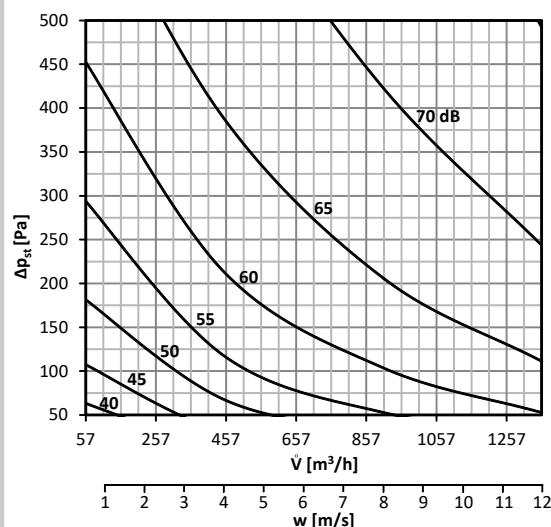
**Graph 10** Sound power level  $L_{WA}$  [dB(A)] inside the pipeline DN225
