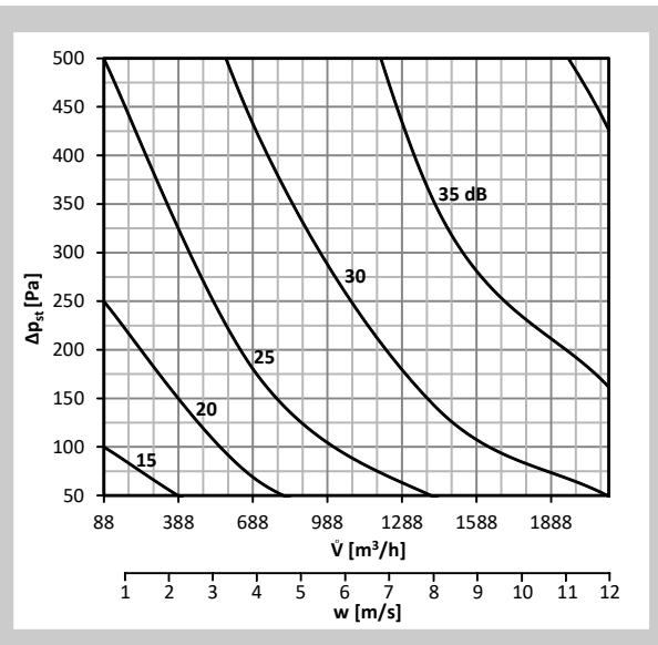
**Graph 34** Sound power level LWA [dB(A)] radiated outside the pipeline DN280, with insulation
