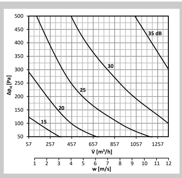
**Graph 32** Sound power level LWA [dB(A)] radiated outside the pipeline DN225, with insulation
