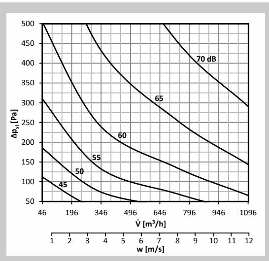
**Graph 9** Sound power level  $L_{WA}$  [dB(A)] inside the pipeline DN200
