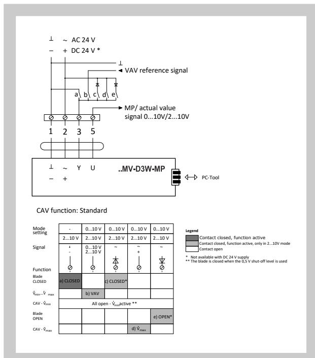
Fig. 12 Master-slave flow control with actuators LMV-D3W-MP.1 MDK
