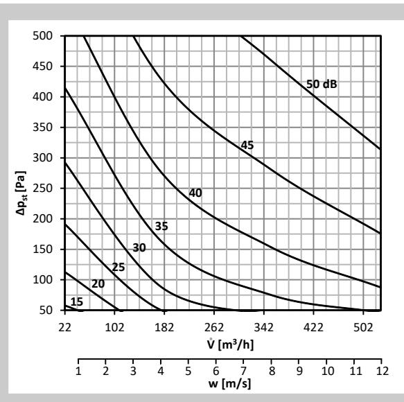
**Graph 18** Sound power level LWA [dB(A)] radiated outside the pipeline DN160, without insulation
