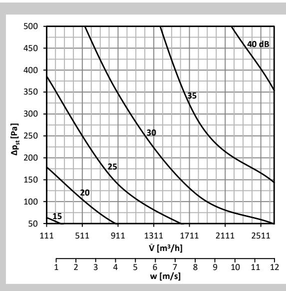
**Graph 35** Sound power level LWA [dB(A)] radiated outside the pipeline DN315, with insulation
