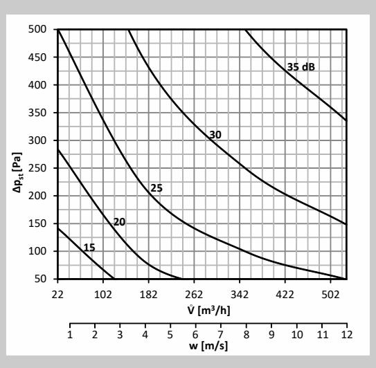
**Graph 28** Sound power level LWA [dB(A)] radiated outside the pipeline DN140, with insulation
