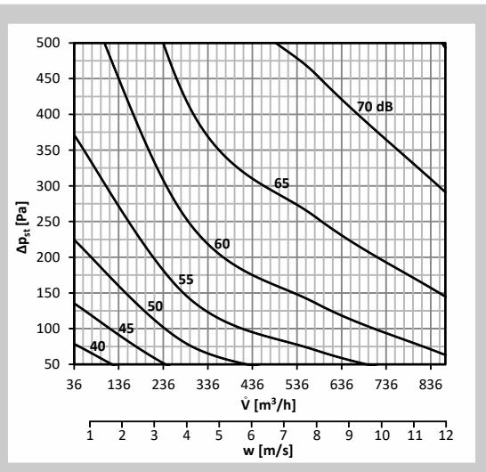
**Graph 4** Sound power level  $L_{WA}$  [dB(A)] inside the pipeline DN100
