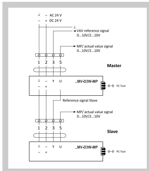
Fig. 13 Controller with BELIMO compact VAV controller LMV-D3W-MOD.1 MDK
