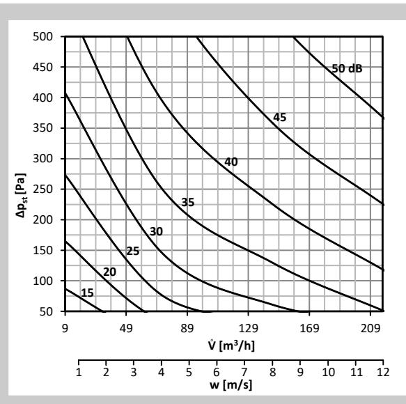
**Graph 16** Sound power level LWA [dB(A)] radiated outside the pipeline DN125, without insulation
