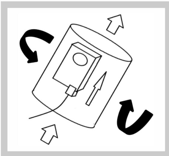
**Fig. 7 Any rotation of the elbow downstream possible**
