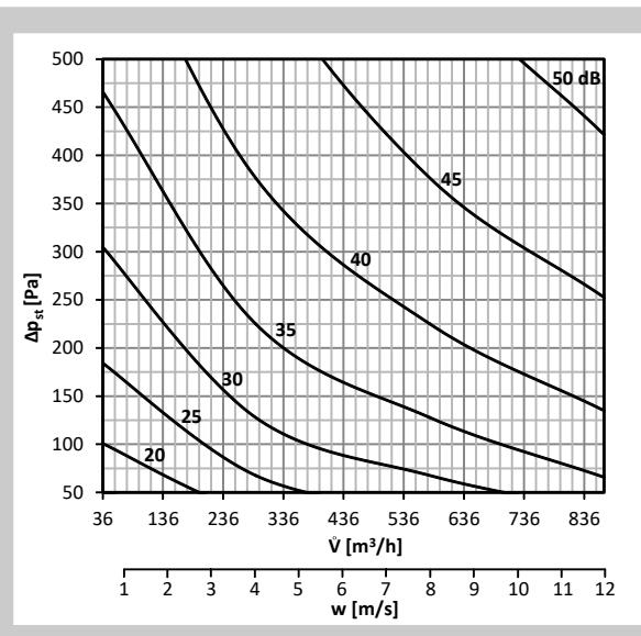
**Graph 15** Sound power level LWA [dB(A)] radiated outside the pipeline DN100, without insulation
