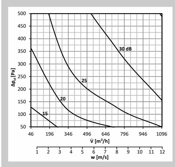
**Graph 31** Sound power level LWA [dB(A)] radiated outside the pipeline DN200, with insulation
